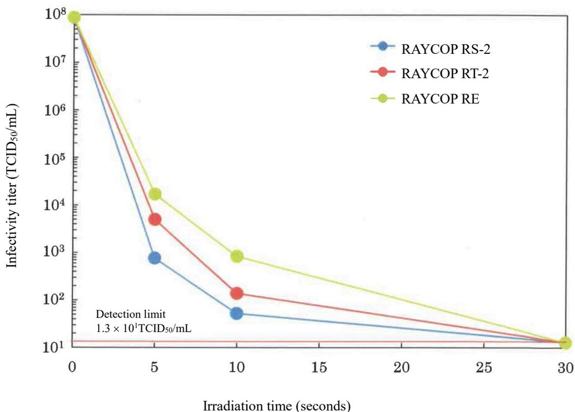
Fig. 2. Test of viral inactivation by UVC lamp built into Futon Cleaner
